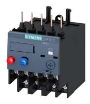
Overload relay 0.55...0.80 A Thermal For motor protection Size S00, Class 10 Contactor mounting Main circuit: Ring cable lug Auxiliary circuit: ring cable lug Manual-Automatic-Reset
