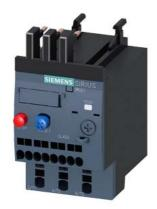
Overload relay 0.55...0.80 A Thermal For motor protection Size S00, Class 10 Contactor mounting Main circuit: Spring-type terminal Auxiliary circuit: spring-type terminal Manual-Automatic-Reset
