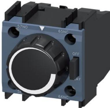
pneumatically time-delayed auxiliary switch, off delayed 1-30 s, 1 NO + 1 NC, for mounting to contactors 3RT202
