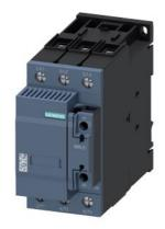
capacitor contactor, AC-6b 75 kVAr, / 400 V, 3-pole, 175-280 V AC/DC, 50/60 Hz, with integrated varistor, auxiliary contacts: 2 NC, screw terminal, size: S2  $\,$
