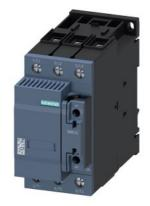
capacitor contactor, AC-6b 75 kVAr, / 400 V, 3-pole, 83-155 V AC/DC, 50/60 Hz, with integrated varistor, auxiliary contacts: 2 NC, screw terminal, size: S2  $\,$
