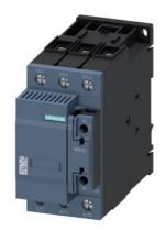
capacitor contactor, AC-6b 75 kVAr, / 400 V, 3-pole, 110 V AC, 50 Hz, auxiliary contacts: 2 NC, screw terminal, size: S2  $\,$
