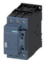
capacitor contactor, AC-6b 75 kVAr, / 400 V, 3-pole, 24 V AC, 50 Hz, auxiliary contacts: 2 NC, screw terminal, size: S2  $\,$
