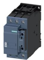
capacitor contactor, AC-6b 75 kVAr, / 400 V, 3-pole, 24 V AC, 50 Hz, auxiliary contacts: 1 NO + 1 NC, screw terminal, size: S2
