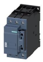
capacitor contactor, AC-6b 50 kVAr, / 400 V, 3-pole, 83-155 V AC/DC, 50/60 Hz, with integrated varistor, auxiliary contacts: 2 NC, screw terminal, size: S2  $\,$
