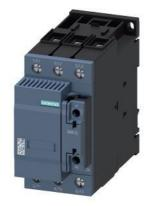
capacitor contactor, AC-6b 50 kVAr, / 400 V, 3-pole, 110 V AC, 50 Hz / 120 V, 60 Hz, auxiliary contacts: 2 NC, screw terminal, size: S2  $\,$
