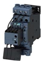
capacitor contactor, AC-6b 33 kVAr, / 400 V, 3-pole, 200-280 V AC/DC, 50/60 Hz, with integrated varistor, auxiliary contacts: 1 NO + 2 NC, screw terminal, size: S0
