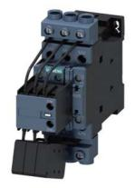
capacitor contactor, AC-6b 33 kVAr, / 400 V, 3-pole, 95-130 V AC/DC, 50/60 Hz, with integrated varistor, auxiliary contacts: 1 NO + 2 NC, screw terminal, size: S0
