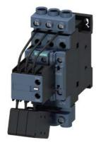
capacitor contactor, AC-6b 33 kVAr, / 400 V, 3-pole, 24 V AC, 50/60 Hz, auxiliary contacts: 1 NO + 2 NC, screw terminal, size: S0
