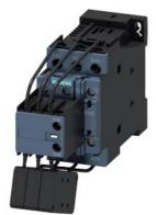
capacitor contactor, AC-6b 25 kVAr, / 400 V, 3-pole, 95-130 V AC/DC, 50/60 Hz, with integrated varistor, auxiliary contacts: 1 NO + 2 NC, screw terminal, size: S0
