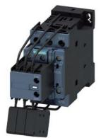
capacitor contactor, AC-6b 25 kVAr, / 400 V, 3-pole, 24 V DC, auxiliary contacts: 1 NO + 2 NC, screw terminal, size: S0
