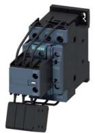
capacitor contactor, AC-6b 25 kVAr, / 400 V, 3-pole, 230 V AC, 50 Hz, auxiliary contacts: 1 NO + 2 NC, screw terminal, size: S0
