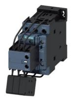
capacitor contactor, AC-6b 20 kVAr, / 400 V, 3-pole, 21-28 V AC/DC, 50/60 Hz, with integrated varistor, auxiliary contacts: 1 NO + 2 NC, screw terminal, size: S0
