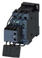
capacitor contactor, AC-6b 20 kVAr, / 400 V, 3-pole, 110 V DC, auxiliary contacts: 1 NO + 2 NC, screw terminal, size: S0
