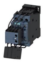
capacitor contactor, AC-6b 16.7 kVAr, / 400 V, 3-pole, 200-280 V AC/DC, 50/60 Hz, with integrated varistor, auxiliary contacts: 1 NO + 2 NC, screw terminal, size: S0
