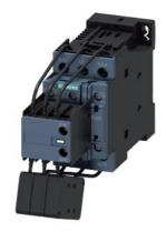
capacitor contactor, AC-6b 16.7 kVAr, / 400 V, 3-pole, 95-130 V AC/DC, 50/60 Hz, with integrated varistor, auxiliary contacts: 1 NO + 2 NC, screw terminal, size: S0
