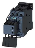
capacitor contactor, AC-6b 16.7 kVAr, / 400 V, 3-pole, 110 V DC, auxiliary contacts: 1 NO + 2 NC, screw terminal, size: S0
