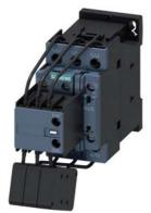
capacitor contactor, AC-6b 16.7 kVAr, / 400 V, 3-pole, 110 V AC, 50 Hz, auxiliary contacts: 1 NO + 2 NC, screw terminal, size: S0
