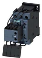
capacitor contactor, AC-6b 16.7 kVAr, / 400 V, 3-pole, 24 V AC, 50/60 Hz, auxiliary contacts: 1 NO + 2 NC, screw terminal, size: S0
