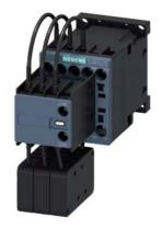
capacitor contactor, AC-6b 12.5 kVAr, / 400 V, 3-pole, 110 V DC, auxiliary contacts: 1 NO + 1 NC, screw terminal, size: S00
