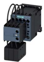
capacitor contactor, AC-6b 12.5 kVAr, / 400 V, 3-pole, 220 V AC, 50 Hz / 240 V, 60 Hz, auxiliary contacts: 1 NO + 1 NC, screw terminal, size: S00
