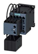
capacitor contactor, AC-6b 12.5 kVAr, / 400 V, 3-pole, 230 V AC, 50/60 Hz, auxiliary contacts: 2 NC, screw terminal, size: S00
