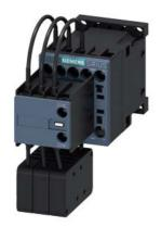
capacitor contactor, AC-6b 12.5 kVAr, / 400 V, 3-pole, 110 V AC, 50 Hz / 120 V, 60 Hz, auxiliary contacts: 1 NO + 1 NC, screw terminal, size: S00
