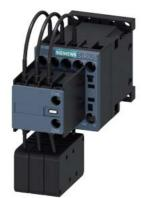
capacitor contactor, AC-6b 12.5 kVAr, / 400 V, 3-pole, 110 V AC, 50/60 Hz, auxiliary contacts: 2 NC, screw terminal, size: S00  $\,$
