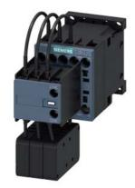
capacitor contactor, AC-6b 12.5 kVAr, / 400 V, 3-pole, 110 V AC, 50/60 Hz, auxiliary contacts: 1 NO + 1 NC, screw terminal, size: S00
