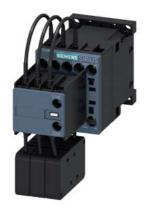
capacitor contactor, AC-6b 12.5 kVAr, / 400 V, 3-pole, 24 V AC, 50/60 Hz, auxiliary contacts: 2 NC, screw terminal, size: S00  $\,$
