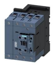
power contactor, AC-3, 80 A, 37 kW / 400 V, 4-pole, 175-280 V AC/DC, 50/60 Hz, with integrated varistor, main contacts: 2 NO + 2 NC, auxiliary contacts: 1 NO + 1 NC, screw terminal, size: S3
