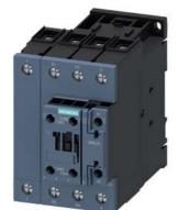
power contactor, AC-3, 40 A, 18.5 kW / 400 V, 4-pole, 175-280 V AC/DC, 50/60 Hz, with integrated varistor, main contacts: 2 NO + 2 NC, auxiliary contacts: 1 NO + 1 NC, screw terminal, size: S2
