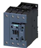
power contactor, AC-3, 40 A, 18.5 kW / 400 V, 4-pole, 83-155 V AC/DC, 50/60 Hz, with integrated varistor, main contacts: 2 NO + 2 NC, auxiliary contacts: 1 NO + 1 NC, screw terminal, size: S2
