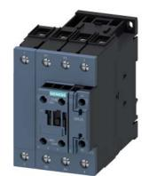
power contactor, AC-3, 40 A, 18.5 kW / 400 V, 4-pole, 220 V AC, 50 Hz / 240 V, 60 Hz, main contacts: 2 NO + 2 NC, auxiliary contacts: 1 NO + 1 NC, screw terminal, size: S2
