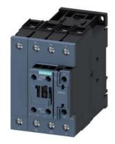
power contactor, AC-3, 40 A, 18.5 kW / 400 V, 4-pole, 230 V AC, 50 Hz, main contacts: 2 NO + 2 NC, auxiliary contacts: 1 NO + 1 NC, screw terminal, size: S2
