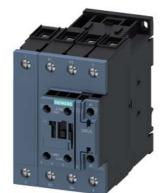
power contactor, AC-3, 40 A, 18.5 kW / 400 V, 4-pole, 110 V AC, 50/60 Hz, main contacts: 2 NO + 2 NC, auxiliary contacts: 1 NO + 1 NC, screw terminal, size: S2
