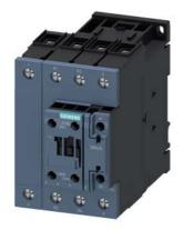
power contactor, AC-3, 40 A, 18.5 kW / 400 V, 4-pole, 42 V AC, 50 Hz, main contacts: 2 NO + 2 NC, auxiliary contacts: 1 NO + 1 NC, screw terminal, size: S2
