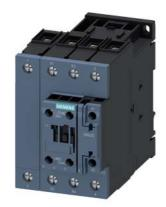
power contactor, AC-3, 40 A, 18.5 kW / 400 V, 4-pole, 24 V AC, 50/60 Hz, main contacts: 2 NO + 2 NC, auxiliary contacts: 1 NO + 1 NC, screw terminal, size: S2
