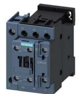
power contactor, AC-3, 25 A, 11 kW / 400 V, 4-pole, 110 V AC, 50/60 Hz, main contacts: 2 NO + 2 NC, auxiliary contacts: 1 NO + 1 NC, screw terminal, size: S0
