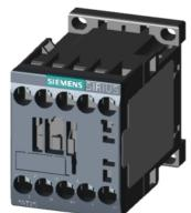
power contactor, AC-3, 16 A, 7.5 kW / 400 V, 4-pole, 110 V AC, 50 Hz / 120 V, 60 Hz, main contacts: 2 NO + 2 NC, screw terminal, size: S00
