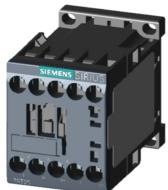
power contactor, AC-3, 16 A, 7.5 kW / 400 V, 4-pole, 110 V AC, 50/60 Hz, main contacts: 2 NO + 2 NC, screw terminal, size: S00
