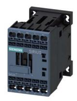
power contactor, AC-3, 12 A, 5.5 kW / 400 V, 4-pole, 220 V AC, 50 Hz / 240 V, 60 Hz, main contacts: 2 NO + 2 NC, spring-loaded terminal, size: S00
