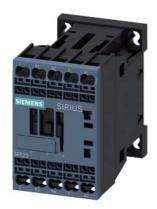
power contactor, AC-3, 12 A, 5.5 kW / 400 V, 4-pole, 110 V AC, 50 Hz / 120 V, 60 Hz, main contacts: 2 NO + 2 NC, spring-loaded terminal, size: S00
