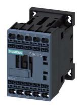
power contactor, AC-3, 12 A, 5.5 kW / 400 V, 4-pole, 110 V AC, 50/60 Hz, main contacts: 2 NO + 2 NC, spring-loaded terminal, size: S00
