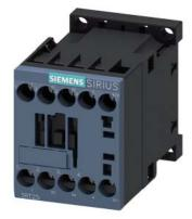
power contactor, AC-3, 12 A, 5.5 kW / 400 V, 4-pole, 24 V DC, main contacts: 2 NO + 2 NC, screw terminal, size: S00  $\,$
