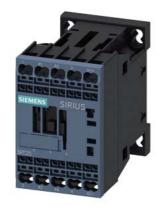
power contactor, AC-3, 9 A, 4 kW / 400 V, 4-pole, 12 V DC, main contacts: 2 NO + 2 NC, spring-loaded terminal, size: S00
