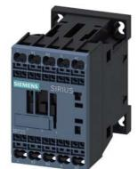
power contactor, AC-3, 9 A, 4 kW / 400 V, 4-pole, 220 V AC, 50 Hz / 240 V, 60 Hz, main contacts: 2 NO + 2 NC, spring-loaded terminal, size: S00  $\,$
