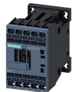
power contactor, AC-3, 9 A, 4 kW / 400 V, 4-pole, 110 V AC, 50 Hz / 120 V, 60 Hz, main contacts: 2 NO + 2 NC, spring-loaded terminal, size: S00  $\,$
