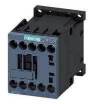
power contactor, AC-3, 9 A, 4 kW / 400 V, 4-pole, 220 V DC, main contacts: 2 NO + 2 NC, screw terminal, size: S00  $\,$
