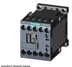
power contactor, AC-3, 9 A, 4 kW / 400 V, 4-pole, 48 V AC, 50/60 Hz, main contacts: 2 NO + 2 NC, screw terminal, size: S00
